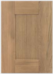
20mm thick, 5 piece, solid Oak frame with veneered MDF centre panel, shaker door with v grooves.
