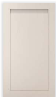
21mm thick, 5 piece, painted solid Ash frame with veneered centre panel, shaker effect door with integrated handle.
