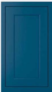
20mm thick, 5 piece, painted solid Ash frame with veneered centre panel, shaker in-frame door with internal bead.
