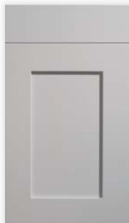
20mm thick, 5 piece, painted solid Ash frame with veneered MDF centre panel, shaker door.
